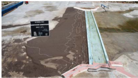
Figure-13. Scouring pattern ( Q = 2400 \text{ m}^3/\text{s} ).
